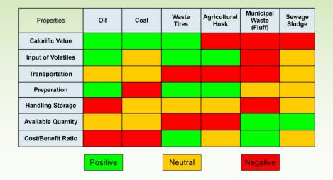
Elaboration of suitable application scenarios based on the physical and chemical properties and commercial aspects whilst considering the particular technology and process requirements of the cement plant and the availability of the AFR.
