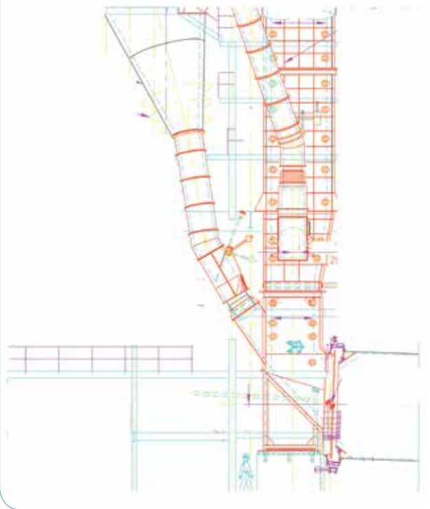
Figure 4. Example of smooth introduction of hot meal via the hot meal slide at the back end of the inlet chamber.
