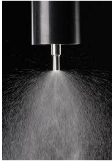
Fig.3: Standard dual media water spray nozzles creating water droplets.
