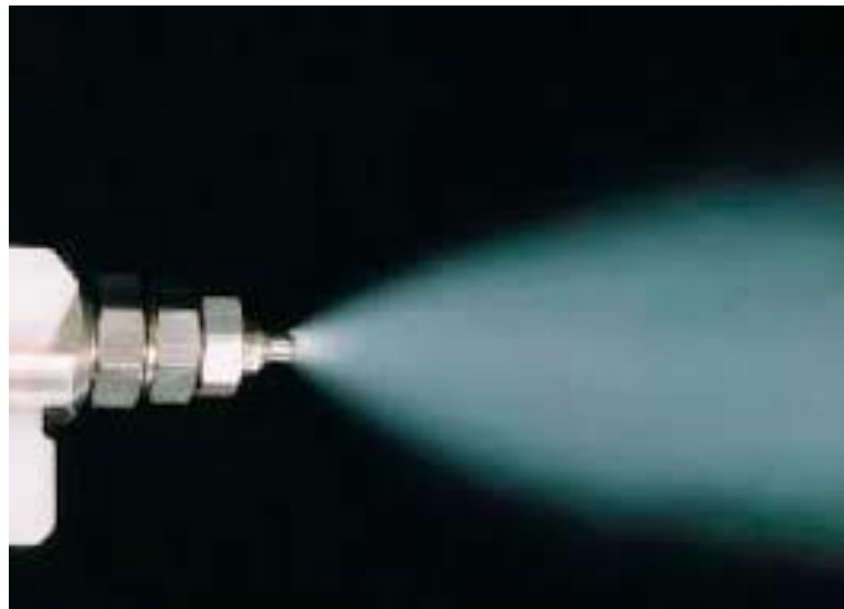
Fig.4: Atomizing dual media nozzles creating a water mist.
